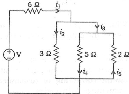
(c) For the given circuit, find  $I_1$ ,  $I_2$  and  $I_3$ , using mesh analysis :
